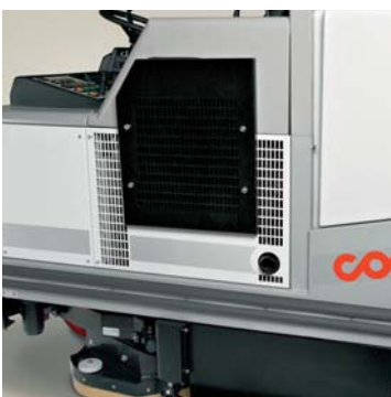
C130 Diesel - Radiator with blowing fan
