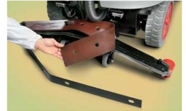
Removing the squeegee rubbers is extremely simple. Just open the hinged clamp with a hammer to easily pull out the rubber
