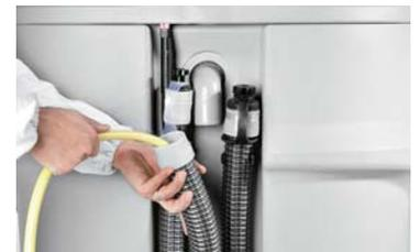
To always ensure perfect floor drying, the squeegee hose should be cleaned at the end of each cleaning session. Thanks to this operation, the suction motor can always operate in perfect conditions and ensure a longer life cycle
